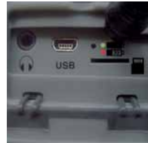
Side door allows quick access to headphone and USB connections, charging port and removable Micro SD card
